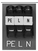
Safe interruption of both supply voltage conductors must be provided for, either by disconnecting the power connector or using a separate switch.
