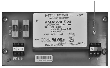
The green LED (3) lights up when the output voltage  $U_{DC} = 24 \text{ V}$ .
