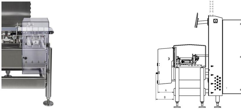
The scale drawing shows Flexus® with a collection container (optional), which is made from plastic (option SSC: the plastic is additional reinforced) or stainless steel – both versions have different dimensions.
